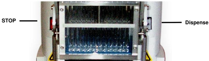
Figure 3-3: Buttons on Either Side of Syringe Array (STOP and Dispense)
