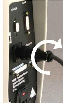
**Figure 2-7: Attaching E-stop plug**
