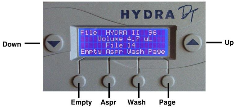
Figure 3-1: Buttons on Operation Screens
