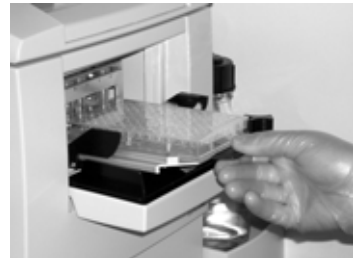
B. Lift out the rack tray.
