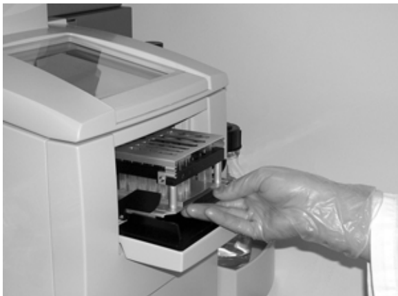
Figure 3-14. Loading the sample and reagent rack into the sample compartment.
