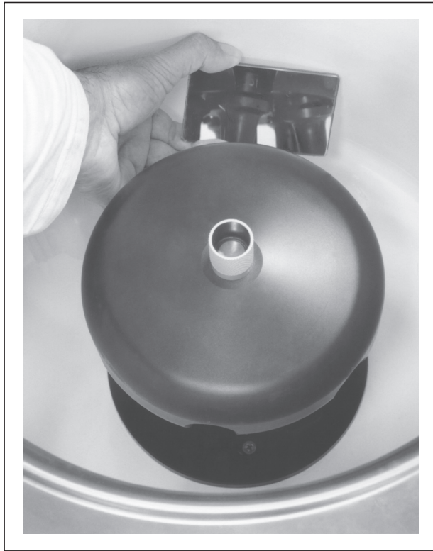
Figure 5.2 Checking Hook-on Bucket Positions After the Rotor is Installed*
